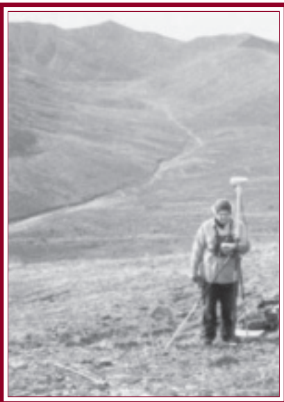
Camp chief Kurt Huhta performing a static observation on a newly established section corner.
