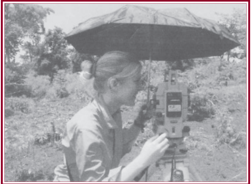
Above: Jean, an eMi intern, takes advantage of some shade while taking field measurements with a Sokkia Set5.
