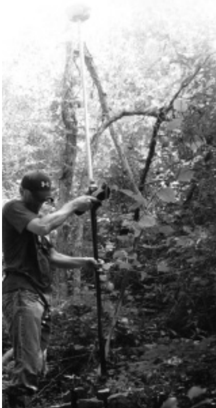
Taking a GPS observation on a U.S. Forest Service monument near Treat, AR.
