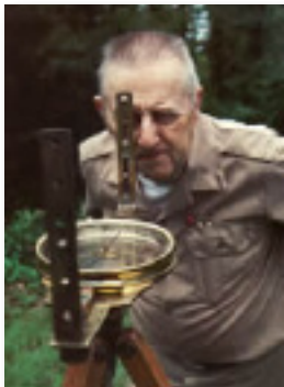
This 1850 Gurley is a brass vernier compass. Mr. Elgin explains how the surveyor would look through the first sight and line the second sight up with the flag pole. This compass is just one of the many instruments that Mr. Elgin has.
