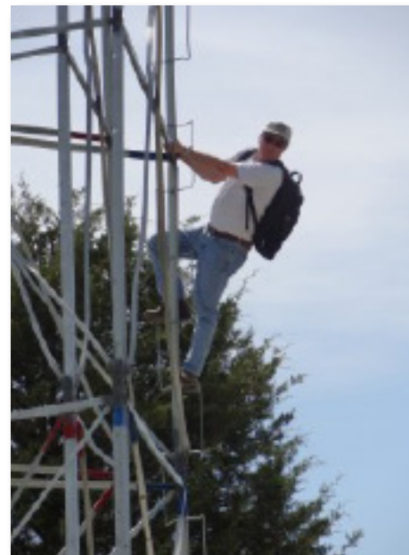
Denny Hoar of the NGS places an antenna on the top to collect GPS data overnight.
