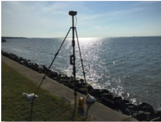
GNSS Receiver measuring a precise static location in Cook Inlet, Alaska.
