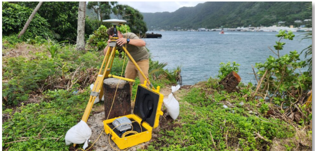
GNSS receiver measuring a precise static location in American Samoa.
