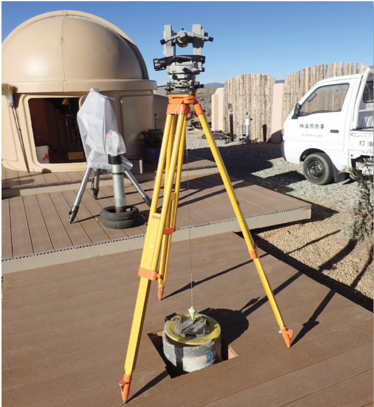
This is the setup with the Sokkia TM-6 theodolite used to set the bearing of the azimuth line from the north property line to the telescope pier. Note the use of a plumb bob even though it had an optical plummet tribrach it was easier to use over the center mark of the bolts on the concrete pier.
