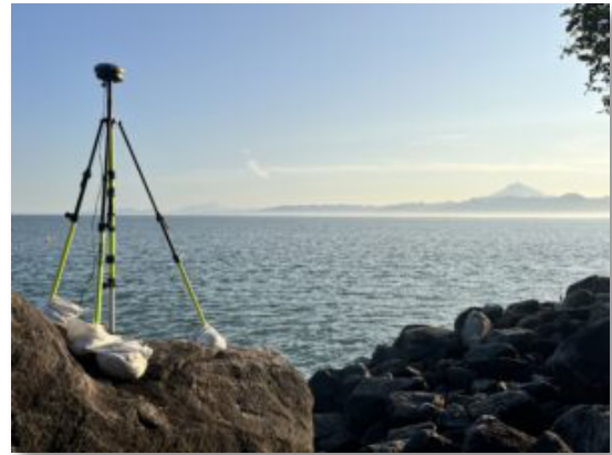
GNSS Receiver measuring ground subsidence in Newport, Rhode Island.
